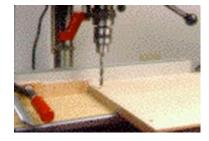
THESE HOLES HOLD IT TOGETHER • If you want your cases to mate correctly, accuracy is key. Use stop blocks on your drill press when drilling the bottom and a doweling jig on the sides.
