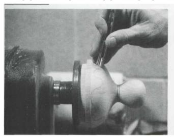
Before removing the parts from the lathe, sketch pencil lines on the lid approximating the shapes to be created. Then with gouges of various sweeps, define those lines (shown above).
