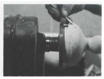
2 Remove material below the line (as shown above), and create the stippled texture by repeatedly tapping a nail set into the surface of the wood.
