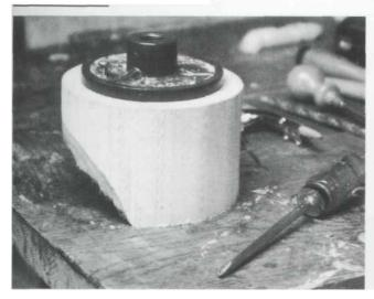
Screw a faceplate to a band-sawn turning blank with large sheet metal screws. Then, install it on the lathe.
