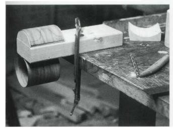
1 This is the bench extension used to maintain the curved form of the sidewall material during the cutting of the lap. The clamping caul is visible on the right.
