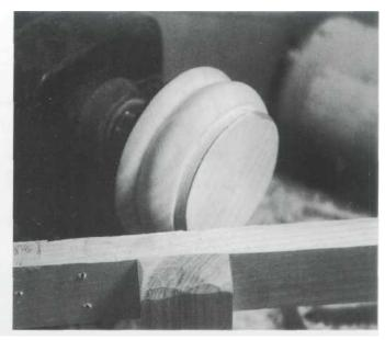
This is the same blank after being turned. Above the bead, notice the flange that will fit inside the box's sidewalls.
