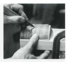
A lap joint is being cut on the bench extension.
