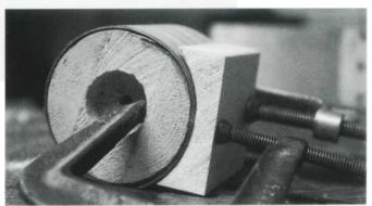
3 Here, the glued lap joint is being clamped with the aid of the caul. Notice that the end of the sidewall material is not positioned under the metal strip as it was during its initial clamping for shape.
