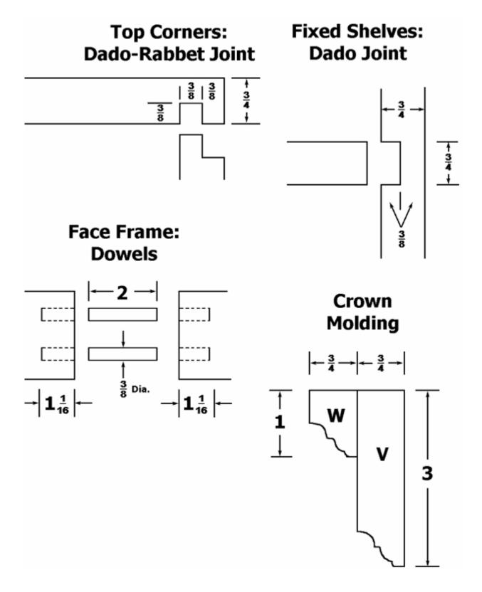
The L-shaped cuts on the top of sides (A, O) are rabbets. Use the same 3/8" adjustment on your Dado blade to cut them 3/8" deep right on the ends of the boards. Notice that these cuts are on the opposite side of the previously cut dados (A, O).
