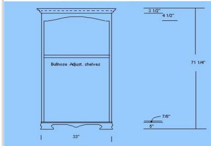
NOTES: Case depth is 12". Stiles and bullnose are 1". A bead is run on the edge of the stile to mate plywood edge, 1/4" cock bead is run on inside opening of bookcase.
