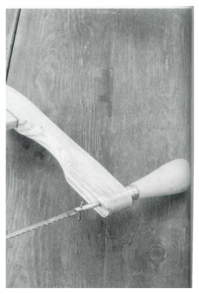
**7** Slide the blade in the slot and fix it in place with a split pin. If at some time you need to fit a slightly longer blade, then you can slide washers on the nail between the ferrule and the cheek.
