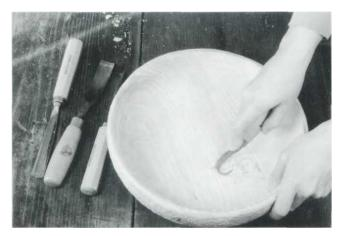
2 One of the easiest ways to bring the bowl to a good finish is to use a hooked sloyd knife. As you are working around the inside of the bowl, be mindful that all along the way you will need to adjust your angle of cut to suit the ever-changing run of the grain.
