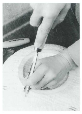
4 The beautiful concave curve shape that runs down from the outside of the foot rim is achieved by thrusting down with the blade and levering back with the handle.
