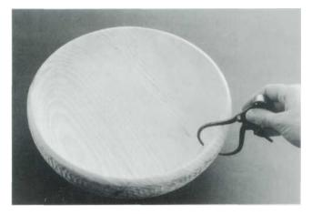
5 All along the way you will have to make repeated checks with the caliper. Try to aim for a section that starts relatively thick at the base and gradually tapers up to a thin rim.
