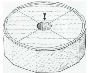
1 Having established the center of the square slab by drawing crossed diagonals and cutting the circular blank, use the 2" diameter Forstner bit to run a 3 1/4-deep pilot hole down into the center (top). Work around the hole clearing the waste (bottom left). Clear the waste level by level, all the while backing up from the pilot hole through to the rim (bottom right).
