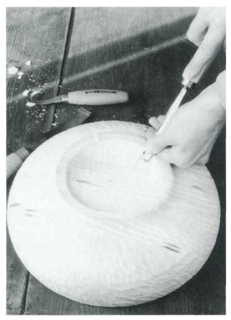
3 When you come to carve the inside of the foot—meaning the inside of the base ring—use small, controlled cuts, with one hand pushing and the other guiding and being ready to break. Notice how in this instance you can lever the shank of the tool on the relatively strong foot rim.
