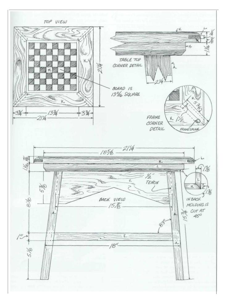
chapter six for a photo of this jig in operation. Please note, however, that in order to cut the slots for the splines on the frame of the chess table, the work would be aligned so that the mitered end of the frame stock sets flat on the saw table). Thickness and cut splines, and assemble the frame
