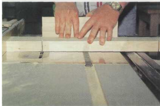
3 Lower the blade to 3/4" and run the backside of the pins to form the joint's cheek.
