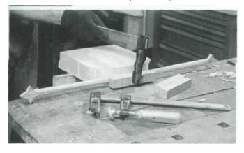
2 Prepare bending forms beforehand. This particular form, a 2"-thick block of poplar cut to the inside profile of the bail, is nailed to a block of wood held in a vise. Necessary clamps and clamping blocks are placed nearby. Gloves are needed because the steamed oak will be very hot when removed from the steam chamber.
