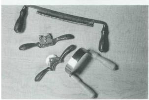
Shown are the shaving tools I use in my shop. The two with turned wooden handles are drawknives. The knife at the top is a general-purpose tool, while the one at the bottom is a variety known as the "inshave" used by makers of Windsor chairs to hollow-out seats. The two middle tools are metal-bodied spokeshaves. The shave with the straight iron is used for general-purpose work, while the other, a hollow shave, can only be used for rounding spindles.
