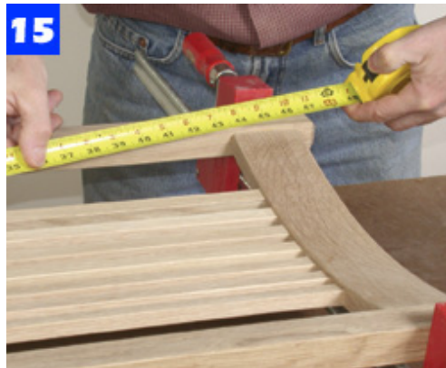
Install slats in the rails. You don't need glue unless the slats are too loose. Then add the remaining rails.
