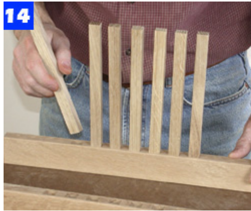
Install slats in the rails. You don't need glue unless the slats are too loose. Then add the remaining rails.
