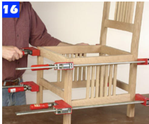
Spread glue and assemble the back frame. Clamp and compare diagonals to check that the assembly is square.
