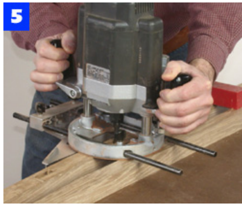
Use a plunge router and edge guide to cut the mortises. Clamp a second leg to the workpiece for extra support.
