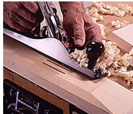
14 -- Use a sharp bench plane to cut long bevels along the top edges of the feet. Then, mark and shape compound bevels.
