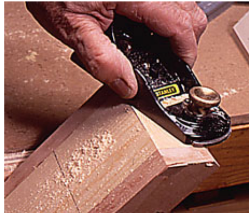
13 -- After cutting foot end bevel with a handsaw, use a sharp block plane to trim the rough-sawn surface smooth.
