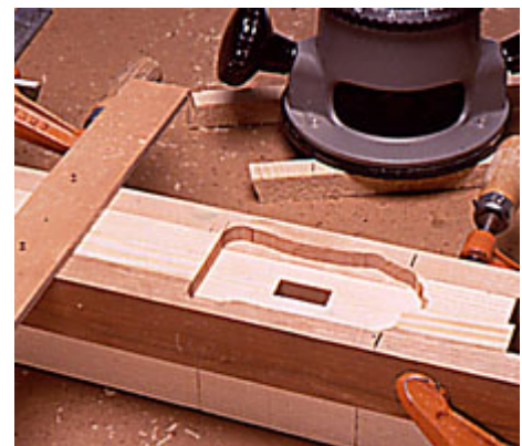
9 -- With the beam halves glued, clamp strips to sides and tack guide strips to edge. Then, rout edges of beam tenon.
