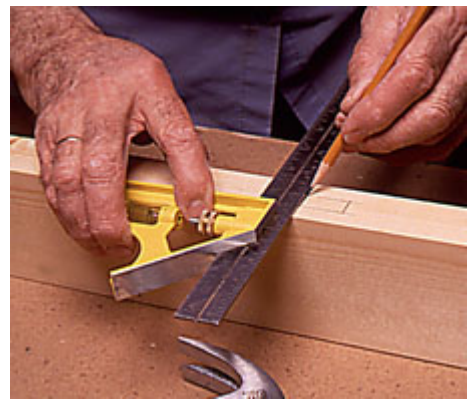
7 -- With the beam halves nailed together temporarily, use a square to lay out the wedge mortises on the beam edges.
