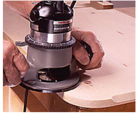
6 -- Use a router and piloted chamfer bit to cut the bevel around the bottom edge of the tabletop. Then, sand the top smooth.
