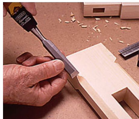
15 -- After routing the stopped bevels on the beam and legs, use a sharp chisel to cut flat, triangular facets at bevel ends.
