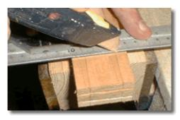
Then you need to place the rail face up in the vice. Score the face line, because you need to cut along that line to remove each face of the tenon and it is cross grain, which is hard to cut. By scoring the line you make it easier to cut.
