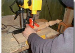
Step Six Cutting the tenons.
