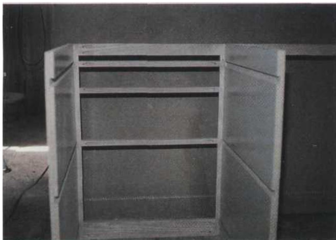
1 Mirrored dados in the drawer bulkheads are ready to receive the drawer shelves.
