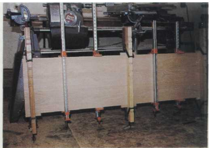
5 Alternating clamps help keep the glued-up top level while drying.
