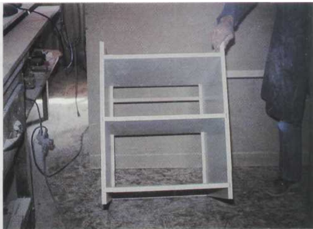
2 The assembled drawer section with shelves in place. The face frame has already been glued on.
