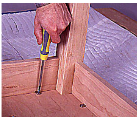
14--Glue and clamp the legs to the rails. Then check for a square assembly by comparing diagonal measurements.
