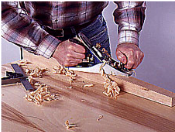
13--Rough cut the leg tapers with a circular saw. Then reduce the edges to finished thickness with a bench plane.
