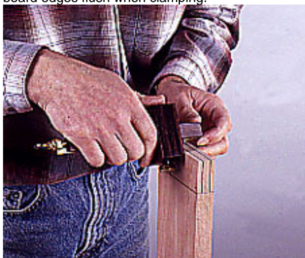
8--Cut the leg stock to size, then apply glue to the mating surfaces. Keep the board edges flush when clamping.
