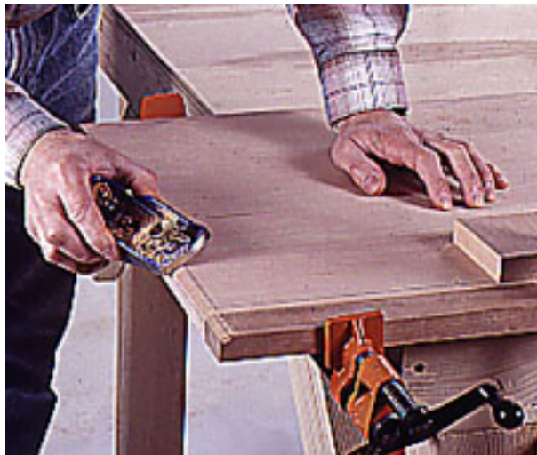
7--Mark the chamfer around the top and plane the edges to this line. A scrap block keeps the side edge from splitting.
