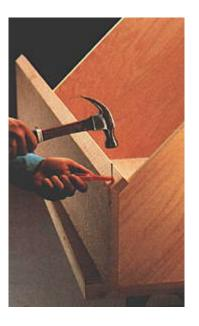
**8.** With table saw blade set to 22  $1/2^{\circ}$ , cut 1  $\times$  2 face frame stiles (as in step 6). Apply glue to the outside edge of each side panel, then attach stiles to side panels using 2" finish nails driven through pilot holes at 8" intervals.
