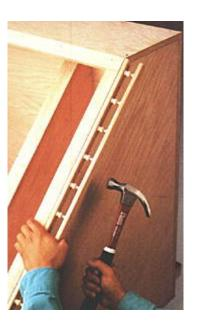
**10.** Measure and cut decorative trim to match the angle of the face frame stiles and side panels, then attach the trim to the outside edges at the top of the cabinet, using finish nails.
