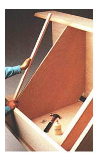
**9.** Measure and cut  $1 \times 2$  face frame rails. Attach them to edges of desktop and top panel, so upper edges of rails are flush with the surfaces of the shelf and top, using glue and 2" finish nails driven through pilot holes.
