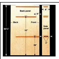
Back panel and side panels have  $1 \times 2$  hardwood cleats to hold the desktop, shelf, and top panel. Attach them to the panels with glue and  $1 \ 1/2$ " screws driven into counterbored pilot holes. Position cleats according to dimensions shown. **NOTE:** If you wish to make the shelf the same size as the desktop, add shelf cleats to the side panels (dotted line).
