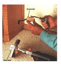
**16.** Sand and finish cabinet then remove plastic. If cabinet will contain electronic equipment, use a hole saw or forstner bit to cut a hole for an outlet strip cord in side panel, then feed cord through hole and install a grommet.
