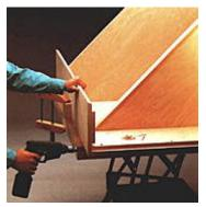
7. Attach 6" cleats to side panels using glue and 1 1/4" finish nails, then attach side panels to back panels with glue and 1 1/2" screws driven into counterbored pilot holes. Cut top panel and attach to cleats with 1 1/4" finish nails.
