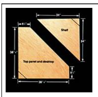
**Desktop, top panel, and shelf** are made from 3/4" finish-grade plywood. Use a circular saw and a straightedge guide to cut the pieces to the dimensions shown. If you plan to use the cabinet as a computer work center or an entertainment center, cut off the back corners of the desktop and shelf (but not the top panel) to provide ventilation and space for routing electrical cords.
