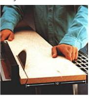
6. Set a table saw blade to 22 1/2° blade angle, then cut 10"-wide, 66"-long side panels, beveling the front edge of each panel.
