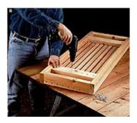
**5.** Position the stretchers between the marks. Drill 1/8" pilot holes through the stretchers into the slats. Attach the stretchers with 2 1/2" screws (**photo B**).
