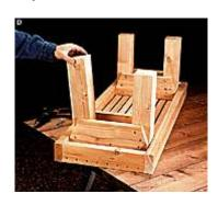
**5.** Position each leg between the braces and against the sides of the bench frame. Drill pilot holes through each brace and attach the leg to the braces by driving 3" screws through the braces and into the leg. Repeat the process for each leg until all legs are installed (**photo D**).
