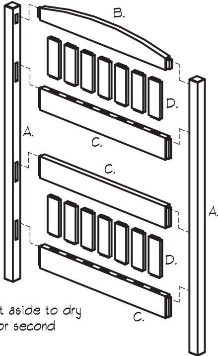
21 Once the slats and rails are assembled, glue them into the mortises on the legs (A.).
