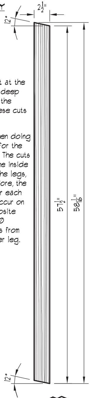
26 Cut a 3/4" wide x 1/2" deep rabbet at the top edge and (4) 3/4" wide x 1/2" deep dados spaced as shown below on the inside face of the ladder legs. These cuts are also made at 12 degrees from perpendicular.
