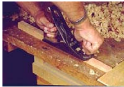
Photo 6- Use a hand plane to make the tapers, or to clean them up after making them on the table saw or jointer. A sharp hand plane is a joy to use, a dull one is worthless. Clamp scraps to your bench as shown to hold the work in place as it is planed.
