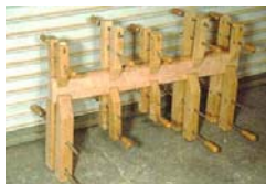
Photo 2- This is the glue blank for the legs. Cleaning the wet glue off this is less important because you can remove dried clumps with the table saw. But, these clumps against the table saw fence make the first cut a pain, so at least smear the wet glue flat if you don't bother to clean it all off. Use a lot of clamps with light pressure rather than a few with a lot of pressure. The number of clamps shown is a minimum for such a glue up.
