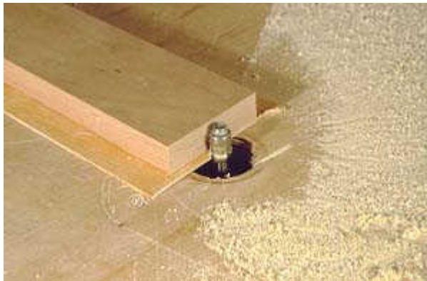
Photo 9- Use a flush trim bit on your router table to flush trim the veneer to the rail edges. Keep your fingers a fair distance from the bit at all times, because the router could grab the work and throw it, pulling your fingers in, especially in a climb cut. See text.
