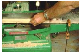
Photo 4- If you have a jointer, tapering the legs is real easy. But- keep your fingers away from the cutter head! Don't pass your fingers over the cutterhead as the cut is made, and always keep your eye on the cut as it is made so you know where your fingers are. See text for proper procedure.
