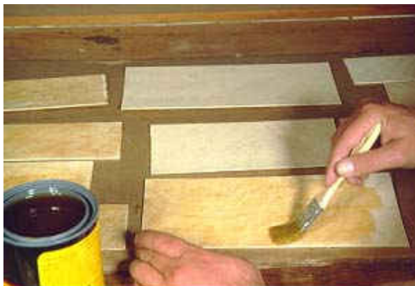
Photo 7- Paint the surfaces to be bonded with contact cement with a throwaway brush. Carefully inspect the areas covered to see if the cement has absorbed completely, or if a thin layer remains behind. If it is completely absorbed, apply more. There must be a thin layer of cement on both bonding surfaces for it to work well.
