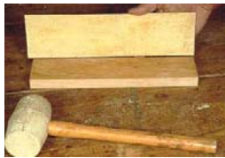
Photo 8- Once the cement has dried, place the veneer pieces on the rails and firmly bang down on all areas with a rubber hammer, or roll over it with a wallpaper roller. Make the veneer pieces larger than the rails, at least 1/4 inch wider all the way around, so it will be easy to locate them on the rails.
