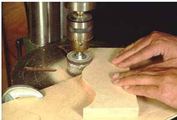
Photo 11- A drum sander in a drill press in a very convenient way to smooth out the curved surfaces. Note that the work rides on a plywood table clamped to the drill press table. This is so the drum bottom can reach below the work, ensuring that the sander hits the entire thickness of the stock.
