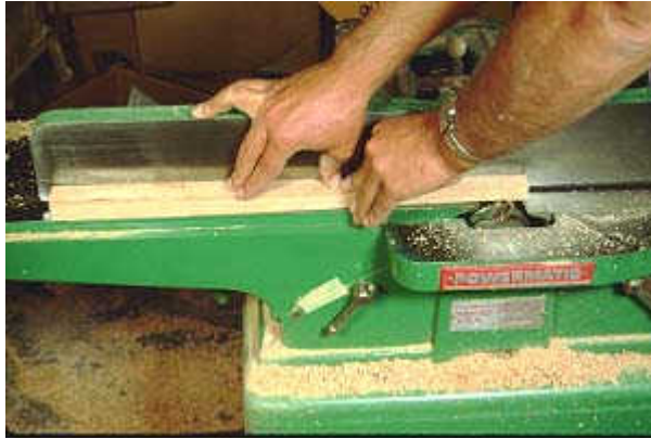
Photo 5- Finishing the taper cut. Having alternately passed your hands over the cutterhead by lifting them above and away from the cutterhead, both hands are on the work again during the final portion of the cut.
