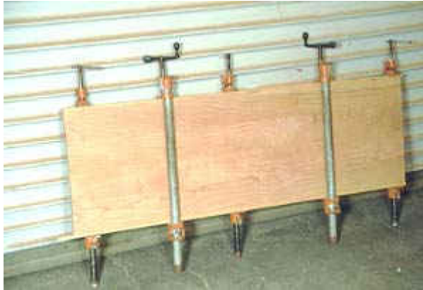
Photo 1- Edge glue your stock to get the widths involved. If you use biscuits or dowels to align the edge joints, be sure you locate them where they won't be exposed after you cut up the piece. Put thin rippings between the clamps and the wood so the clamp doesn't dent the wood. Clean the wet glue off with hot water and a rag. It's harder to clean off after it's hard.
