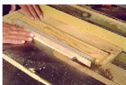
Photo 3- Make this simple taper jig to cut the tapers in all the legs. Be very careful with such a jig. Use a push stick to hold down the leg during the final part of the cut. Don't hold your fingers on the leg
