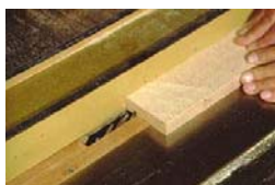
Photo 12- You can use a dado cutter on your table saw to cut the hole drilling plane, or just use your combination blade, taking two passes to end up with a dado 1/4 inch wide.
