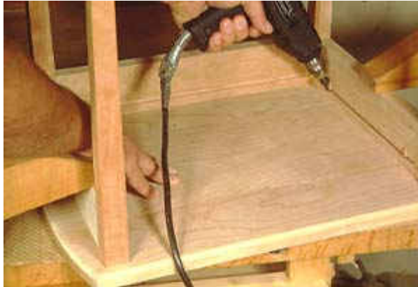
Photo 16- Use a tapered bit with countersink to drill holes for the screws. You don't need the countersink here, but it cuts away some of the wood above the dado to make it easier to get the screw in place.
