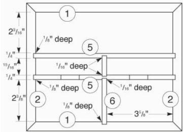
float so that it can adjust to environmental changes.) Clamp box together with <u>web clamps</u>, rubber bands, etc. until glue dries. Remove excess glue with damp rag while glue is still wet.
