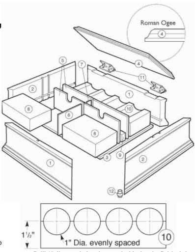
Drill 1" diameter holes, then cut the block to its finished size.
