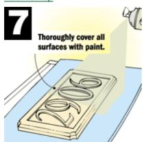
Remove the patterns and sand away any whiskers left by the router. Spray a couple of light coats of paint to seal the wood, followed by one or two heavier coats.
