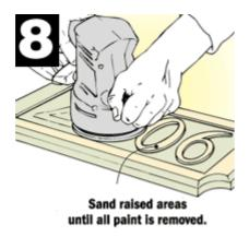
After the paint dries, sand the paint off the raised surfaces to expose the bare wood. Wipe a liberal coat of household bleach on the bare wood, let it dry, then lightly hand sand to remove any raised grain.
