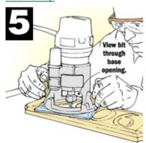
Start routing with the 1/4"-dia. straight bit. If you're working with pine, as I was, you can set the bit for the full 1/4" depth-of-cut. Then ease the bit into the wood anywhere in the area of the field you'll be removing. Rout as close as you comfortably can to the numbers and the edges of the border.
