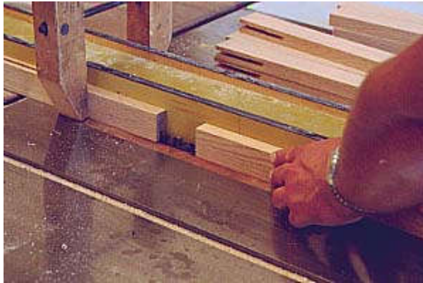
Photo 2- Use this table saw dado setup to cut grooves in the drawer frame fronts and rears to serve as mortises. If you don't have a dado set for your saw, you can use a regular combination blade, just do several setups to get a mortise that is 1/4" wide and centered in the part.
