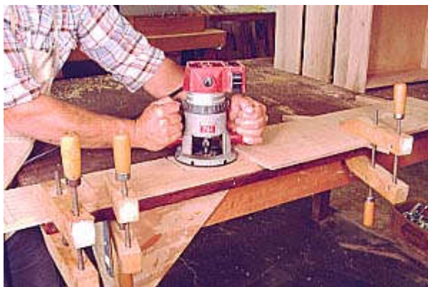
Photo 14- Use this set up to cut the dovetail slots in the top plate as well as the desk sides for the cubbie components. Do a lot of careful measuring to be sure you are centering your slots just where they need to go. Remember that the parts are longer by the dovetail tenons.
