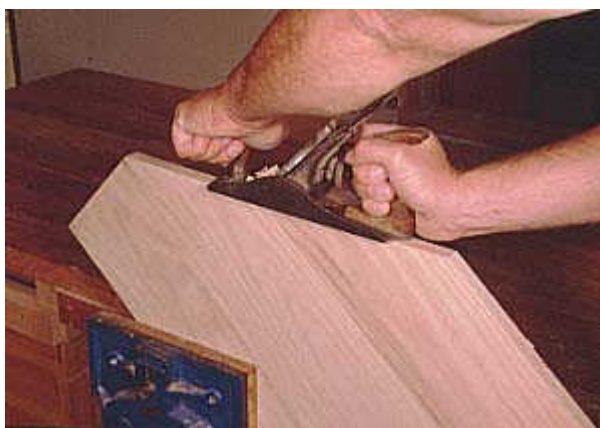
Photo 5- A hand plane will smooth the angled cuts on the desk sides quickly and easily. It will do the same for all edges, though a block plane works best for end grain (that's what they were made to do). If you don't have a hand plane a belt sander will do the job, or a stationary belt or disk sander, or hand sanding, though this alternative will take time. A hand power plane will work well here too.
