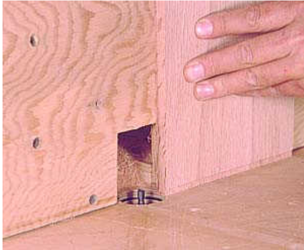
Photo 13- Cut the dovetails on the ends of parts for the drawers and cubbies with a router table setup like this. Having stock of very uniform thickness will help a lot to make uniform dovetail tenons that fit the grooves consistently.
