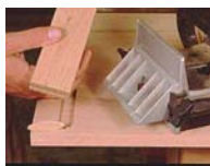
Photo 10- Use a biscuit joiner to locate biscuit splines for the top and bottom rails. Or, use a dowel jig for dowel holes in the rail end, and set up with a drill press to bore dowel holes in the desk sides. If you don't have a drill press, make a wood drilling guide by boring a hole of the dowel size you will use in a thick chunk of scrap. Align this chunk on the desk side so that when the drill bit is placed in it, the bit will be aligned correctly for the dowel. Use this to bore the dowel holes.
