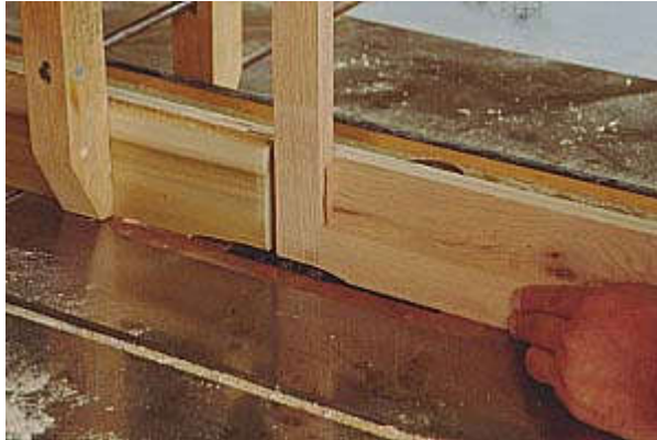
Photo 9- A dado set makes the cut fast, easy and accurate since it cuts to a very even line and is easy to adjust for depth. Make test cuts on scrap to be sure you don't cut too deep, making a visible gap on the front of the drawer frame.
