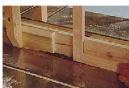
Photo 8- Use this setup to put a stopped dado in the front corners of the drawer frames. If you don't have a dado set for your table saw, these cuts can be made with a band saw or by hand.
