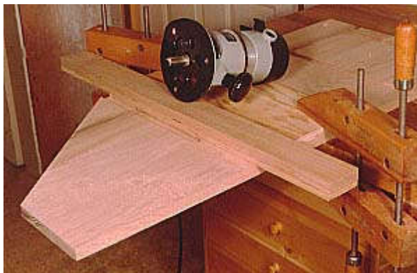
Photo 7-Your fence height and height of the overhead bearing flush trim bit need to be coordinated so that the bearing hits wood and the bit cuts the dados at the correct depth, 1/4". This may be easier to attain with a template guide and straight bit, but such a setup is a little trickier to align due to the offset of the template guide from the bit.
