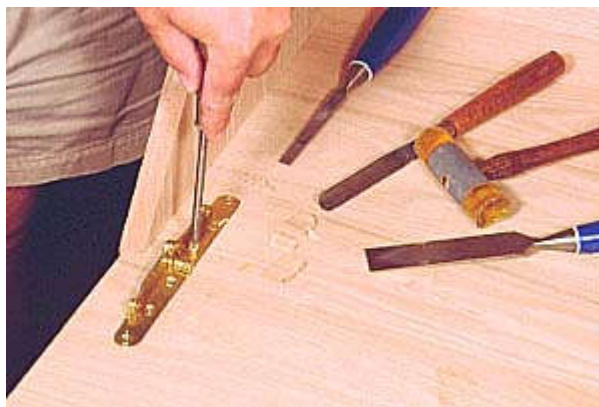
Photo 15- Desk lid hinges are designed to hold the lid open firmly in a horizontal position.
