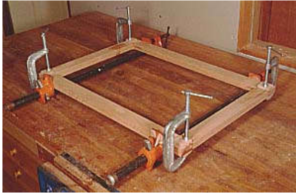
Photo 4- Glue up the drawer frames. Before you put on the C-clamps, check to see that the frame is square by putting your tape on the diagonals across far corners. When these two measures are equal, the frame is square.
