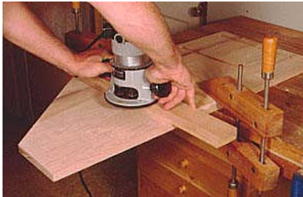
Photo 6- Cutting the dados in the desk sides with an overhead bearing flush trim bit. The bearing rides against the wood fence which is attached to a piece of plywood. The plywood is clamped to the desk side and bench with handscrews as shown. You could also use a straight flute bit and template guide in the router for this operation.
