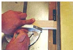
Photo 3- Cut tenons on the ends of the drawer frame runners using your miter gauge at the table saw like so. Again, you don't need to use a dado set here, you can make the cuts with repeated passes using a combination blade.
