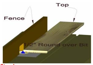
**Step 1:** Once the base has been cut from the top piece, rout the ends of the top.
