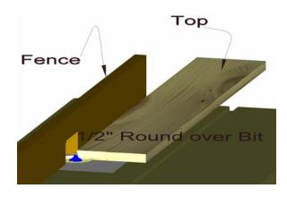
**Step 1:** Set the router fence in line with the round over bit bearing. Raise the bit to the edge of the sink shelf top. Rout the long sides of the top only.
