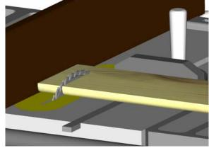
**Step 2:** Make a mark on the top piece at 1 1/2" from the edge. Cut two pieces measuring 1 1/2"; this will make the 2 pieces that make up the base on each side.
