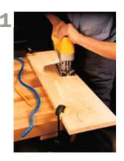
When you're riding your jigsaw around the curves, guide the blade smoothly so you don't create bumps and dings that you'll have to sand out later. Many jigsaws have a dial that allows you to adjust the stroke of the blade to be either gentle or aggressive, depending on the wood you're manipulating and the mood you're in.
