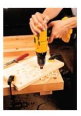
Plug-cutters come in different sizes and varieties. I used a ½" tapered bit to cut my plugs. The resulting plugs are slightly narrower at one end, which makes them easier to push into the hole later. One safety tip: To prevent the plug-cutter bit from bucking and skating on the wood, set the teeth of the bit in the wood by leaning heavily on your drill before you begin. Then keep some weight on the drill as you start the motor.
