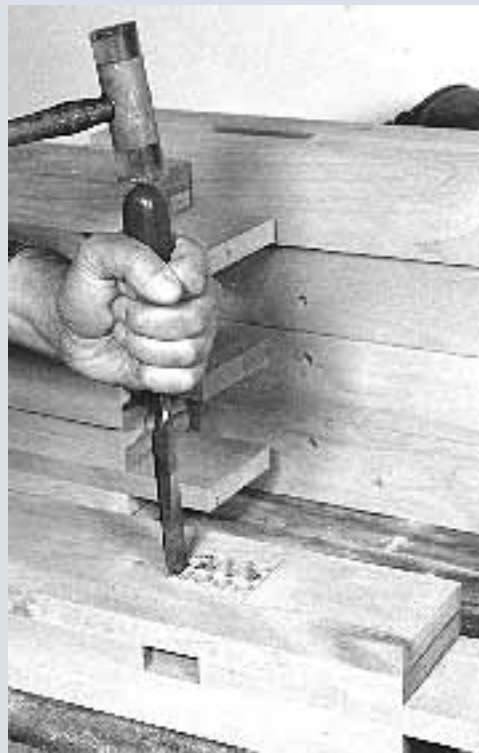
Photo 6- Cut mortises in the posts for the lower stretchers. Mark out the mortises, bore holes within the marks, then clean out the waste with chisel and hammer.
