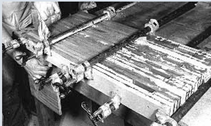
Photo 5- Gang clamp the laminations together, then use very hot water to remove as much glue as possible from the outside of the pieces, as well as within the mortises.
