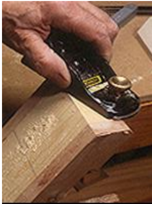
13. Use handsaw to cut foot end bevel and sharp block plane to trim the rough-sawn surface smooth.
