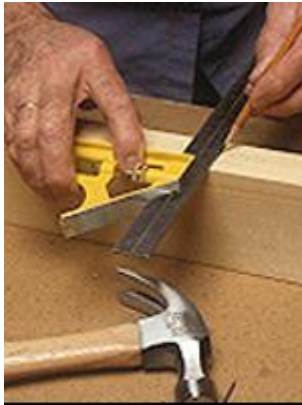
7. With beam halves nailed together temporarily, use square to lay out wedge mortises on beam edges.
