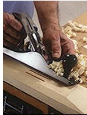
14. Cut long bevels along the top edges of feet with a sharp bench plane, then mark and shape compound bevels.
