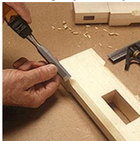
15. After routing stopped bevels on beam and legs, use sharp chisel to cut flat, triangular facets at bevel ends.
