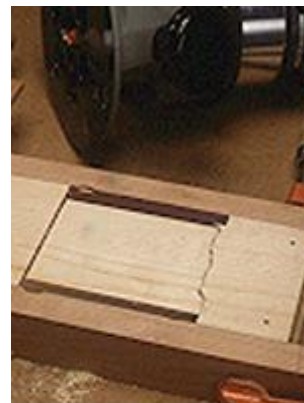
10. Repeat the process on faces of beams to finish tenons. Make tenons slightly longer than finished length.
