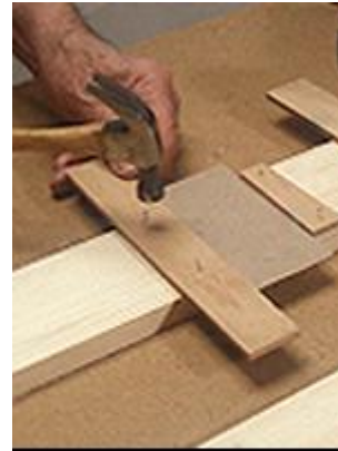
8. With plywood mortise template in place, use cardboard spacer to position router guide strips on one beam half.
