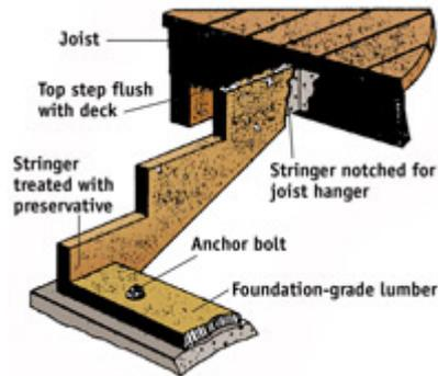
**FIG. 6** - Stringers may be hung from the rim joist with a joist hanger so the first step is flush with the deck surface. In this configuration, a piece of pressure-treated lumber is bolted to the landing pad and the stringer is nailed to it with 16d galvanized nails. From the Sunset book, *Decks*, © Sunset Publishing Corporation.
