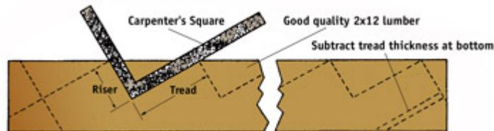
**FIG. 5** - Set the carpenter's square on the stringer so the riser and tread dimensions are at the edge, then trace along the square. Move the square to the previous mark and repeat the process. Subtract one tread thickness from the layout at the bottom so the last step is equal in height to the rest. From the Sunset book, *Decks*, © Sunset Publishing Corporation.
