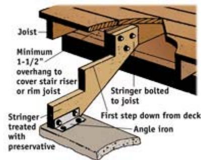
**FIG. 7** - The stringer can be bolted to the end of the joist so the first step is one step below the surface of the deck. At the landing pad, the stringer may be fastened to an angle iron (the angle should be galvanized) bolted to the concrete. From the Sunset book, *Decks*, © Sunset Publishing Corporation.
