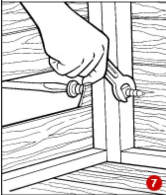
The action of tightening the screws or banging home the nails draws the wall panels together (7). Subsequent panels are secured to each other.
