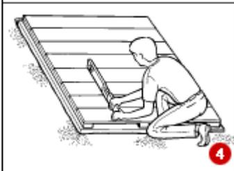
The floor will comprise boards fixed to bearers. It is simply laid in place and will be held there by the weight of the shed. Check with a spirit level that the base is horizontal (4).
