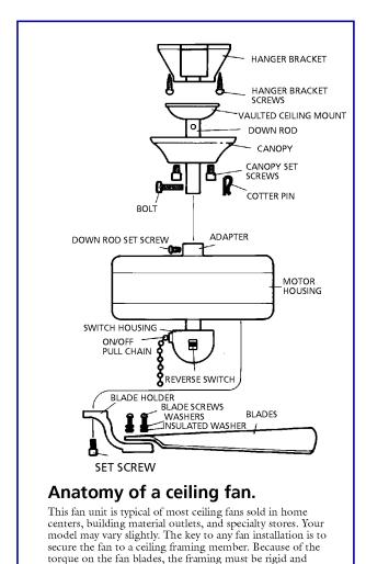
solid. The hanger bracket attaches to the framing and the
