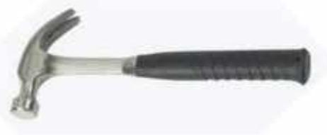
The claw can be used to lever up floorboards or where other places where a lever is required; care must be taken (especially with cheaper models) as the force applied can easily weaken the joint between the handle and the head.
