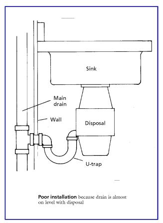
If this doesn't do it, remove the trap along the drainpipe and clean it. Also, with an auger or plumber's snake, rod out the drain from the trap through the drain pipe—not back up through the disposer. Never pour liquid drain cleaner down through the disposer to open a slow or clogged drain. You could damage the disposer.
