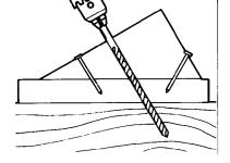
To drill angles, make an angled block to specifications. Then drill through block into work. Block offers support and guides drill bit.
