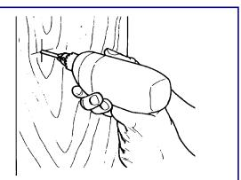
Hold housing of drill this way on horizontal surfaces, applying pressure to back of drill and guiding drill with hand that holds
