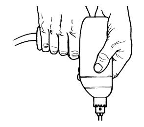
**Support drill** this way when drilling vertically into surfaces, applying pressure on housing not handle. Start drill slowly; then increase speed.
