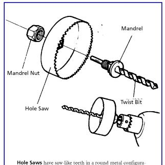
tion. A drill bit in a mandrel guides the saw in material as
