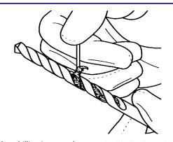
When drilling into metal, remove the drill bit often and clean the metal shavings from the webs and lands of bit. Protect your hands with work gloves and use oil for lubrication.
