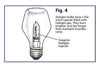
Caution: Don't use halogen bulbs in wet locations. Unlike incandescent lamps, they may continue to light after the bulb has been damaged from exposure to moisture or physical abuse. The inner glass capsule operates at high temperature and pressure, which could lead to sudden shattering.
