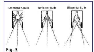
The advantages of R and ER lamps over standard incandescent for specific lighting uses.
