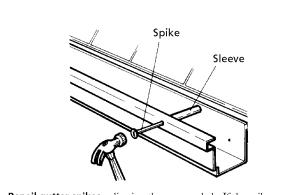
**Renail gutter spikes**, adjusting them as needed. If the spike cannot be removed, cut it off with a hacksaw and drive in a new one. Then, with pliers, adjust the spike/ferrule for right pitch.
