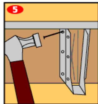
6. Take the short piece of joist material and put it in place in the open joist hanger.
