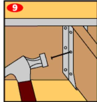
10. Where each joist crosses the beam, screw or toe-nail the joist to the beam. The deck frame is now complete. It is time to proceed with decking and railings.
