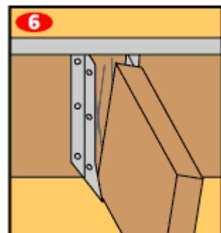
7. Flex the joist hanger up tight against the board. Make sure the top of the board is flush with the ledger of header joist. Nail the other side of the joist hanger in place. Repeat the last 2 steps until all the joist hangers are in place.
