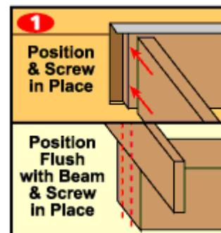
2. Measure and cut the header joist. Position it across the ends of the outside joists and screw it into the ends of the outside joists.
