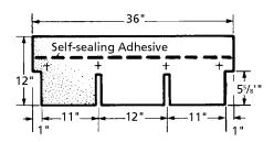
**Always use 4 nails** to fasten on shingles. The Xs mark the spots. The center nails are directly above the cutouts for three tabs, or 11 ins. from the outside nails. Some shingles are marked for nail locations. If not, measure.
