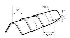
This is the preferred nailing (or stapling) locations for shingles applied to ridges and hips of roofs. Use one fastener on each side, as shown. The exposure remains at 5 inches, same as the exposure of field shingles on the roof.
