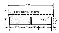
For 2-tab shingles, four nails are still used to fasten them in place. The nails are 5-5/8 ins. from the bottom, or halfway between the sealant and the cutouts. Use zinc-coated fasteners and drive them straight in.
