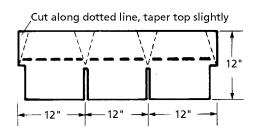
To create your own hip or ridge shingles, mark and cut a regular shingle to fit. Apply the shingles from both roof sides; then finish intersection. Bend ridge shingles lengthwise so they extend equal length down roof sides.
