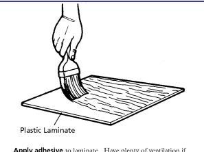
**Apply adhesive** to laminate. Have plenty of ventilation if adhesive is the solvent type.
