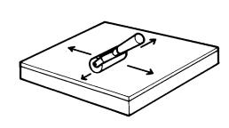
**Roll laminate** so its entire surface touches the core material. Or you can use a hammer and buffer block of wood to tap the laminate tight to the core.
