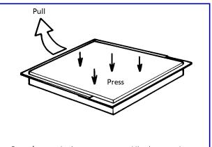
Press down on laminate as paper or molding is removed. Once surfaces of core/laminate touch, the laminate can't be moved or reset on the core.
