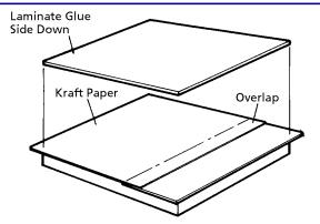
**Separate surfaces** with sheets of kraft paper or lengths of molding. Then align laminate with the core material and remove paper/molding for bond.
