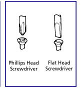
Remember to always fit the blade of the screwdriver to the slot of the screw. Do not use over- or under-sized blades, or the wrong blade in the wrong screwhead, such as a standard blade in a Phillips head or crosshead screw. If the blade is too big or small for the screw slot, you can damage the slot so the screw can't be either driven or drawn. If the blade is too wide, and it sticks out around the screw slot, the blade can damage the material surrounding the screw.
