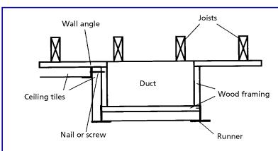
**Piping or ductwork** can be boxed in using a combination of the grid system and framing. Simply nail or screw through the wall angle and tile into the wood frame.
