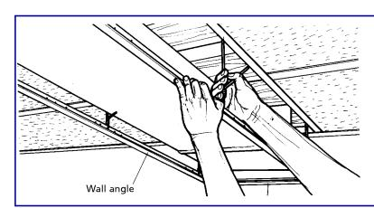
Hang runners below the obstruction from wires attached above the edges of the main ceiling. Use chalkline to mark the level. Attach the runners to wall angle with pop rivets through predrilled holes where they meet the wall.
