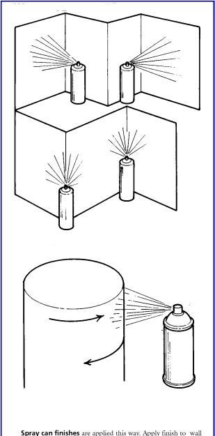
**Spray can finishes** are applied this way. Apply finish to wall or adjoining surfaces first. Then spray the corners. Finish outside corners after adjoining surfaces. Go around rounds.
