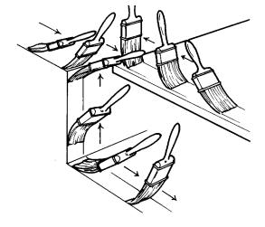
Here's how to apply finish to flat surfaces, and outside, and inside corners. Reverse the brush as indicated by the arrows.
