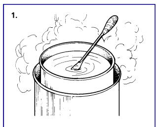
Making pick stick for dust and debris is easy. Heat varnish in "double boiler" using tin can and a pan for utensils. Varnish does not have to boil, just warm it enough to dissolve the chunks of rosin. Dip swab into the mixture.
