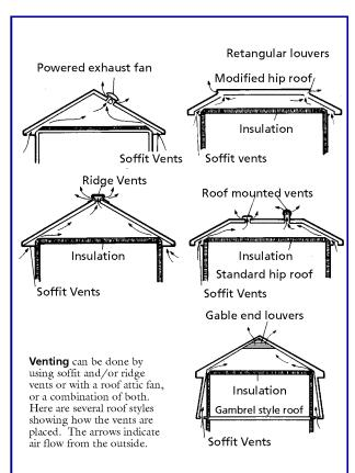
How to ventilate attics. Natural ventilation relies on fixed non-powered devices called ventilators, or "vents." These are located in openings in the attic—or other space to be ventilated—to take advantage of the natural flow of air. Cool air enters the lower vents, is warmed, then rises and moves out the upper vents to expel both heat and humidity.
