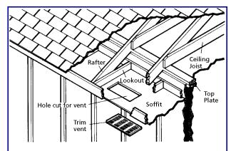
**Rectangular louvers** are inserted into the soffit at the overhang of the roof. The soffit usually is 1/4-in.-thick plywood or sheet material that is easily cut with a sabre or keyhole saw. The louvers are simply inserted into the cut hole and fastened with nails or (usually) screws. Wear safety glasses while sawing the holes.
