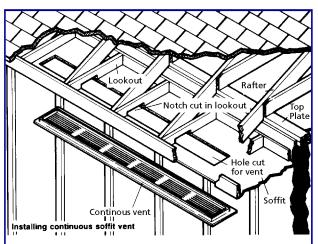
**Continuous soffit** vent is installed the very same way as a rectangular one, except that the lookouts have to be notched with a chisel to "let in" the vent so it fits flush with the surface of the soffit. You can use a sabre saw for this cut but use a blade that won't cut deep into the lookouts.
