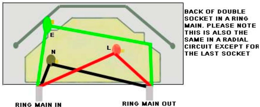
The other type of circuit used to power your home is a radial circuit. There are not so common and can easily be turned into a ring circuit. See our project on [radial circuits](#).
