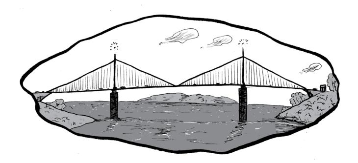
Triangles, the simplest polygons, have some very useful characteristics. Triangles often appear in structures that need to be very strong, like bridges and building frameworks. Why? Three beams connected in a triangle can form only one shape. In contrast, four beams connected in the rectangle can form more than one shape. If you put enough weight on one side of a rectangle, you can smash it into a parallelogram.
