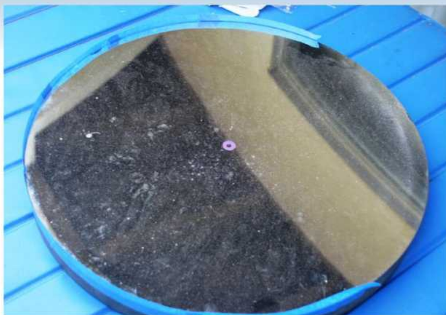
If the mirror in your reflector looks like this, cleaning it will enable it to gather more light. It will also scatter less of the light it collects and perform much better. ROB HAWLEY
