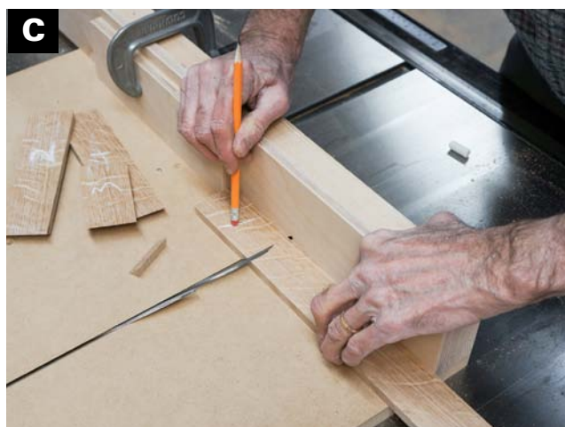
USE THE SPACER BLOCK to shorten the distance between the stop block and blade as you cut the ends.
