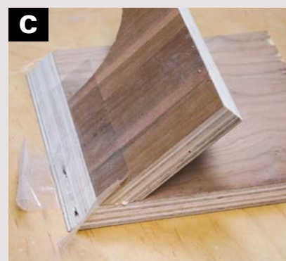
ALLOW THE ASSEMBLED JIG to rest with the parts in position as the glue dries. Wait 45 minutes before using brads, pins, or screws to permanently position the parts.
