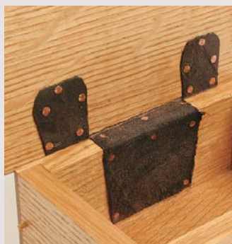
Three pieces of leather—two end pieces and a center piece—are secured with brass tacks to create a unique hinge.
