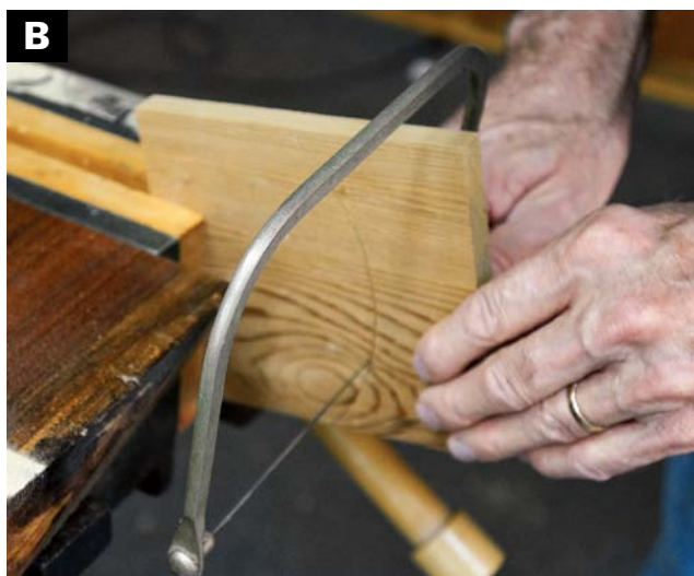
USE A COPING SAW to make the curved cut.
