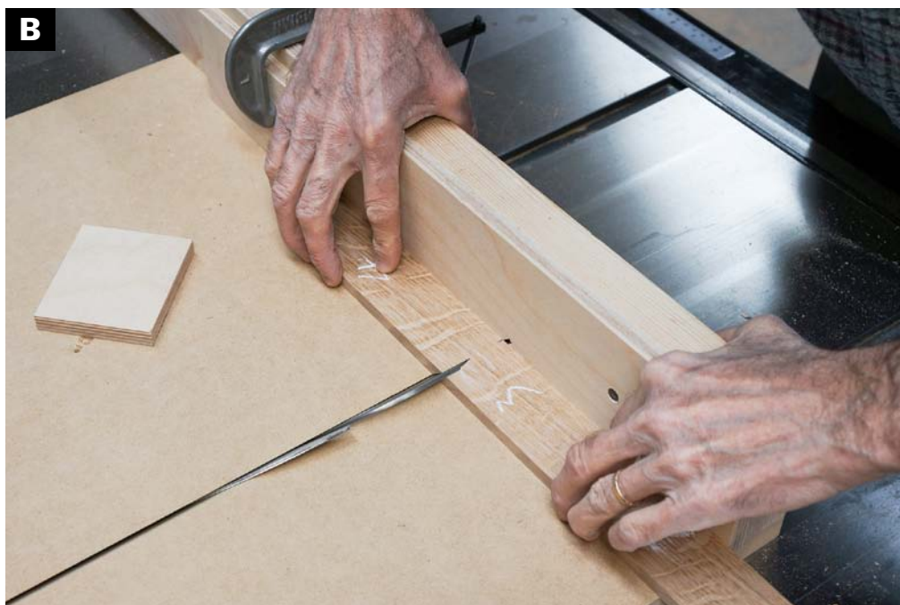
HOLD THE WORKPIECE firmly against the stop block to cut the first mitered part. Note the 3½-in.-long spacer block that will be used for the alternating cuts.
