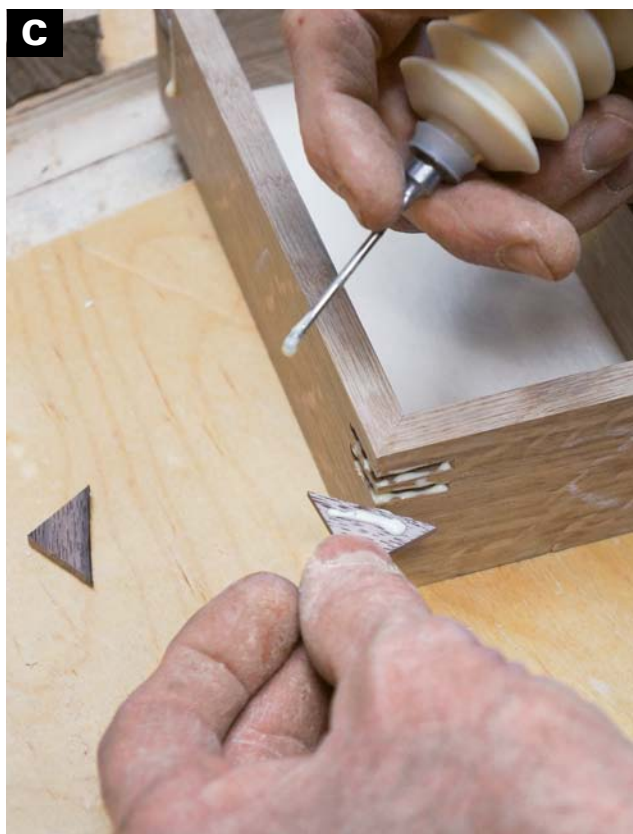
SPREAD GLUE in the key slots and then individually on each key as it is pushed into place.
