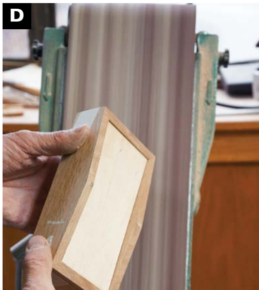
SAND FLAT SURFACES , where possible, using a stationary belt sander or flat sanding sheet.
