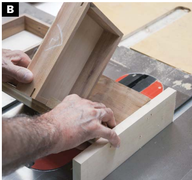
CUT KEYED MITER slots on the tablesaw. A spacer block is used in the keyed miter guide to hold the box in the right position for each cut.
