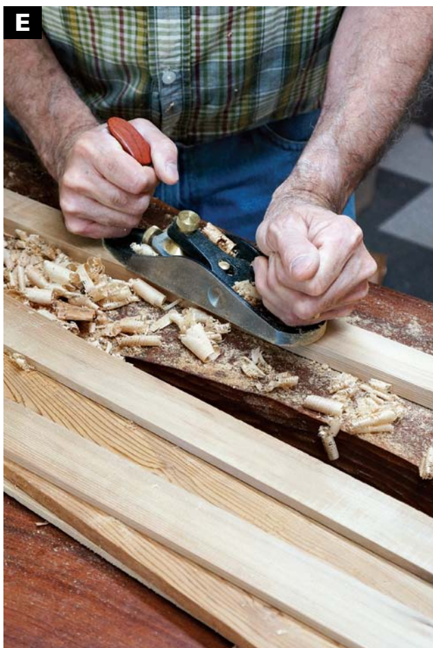
PLANE THE MATERIAL for the front, back, and ends smooth, making each piece uniform in thickness. Minor variations in this box are OK.
