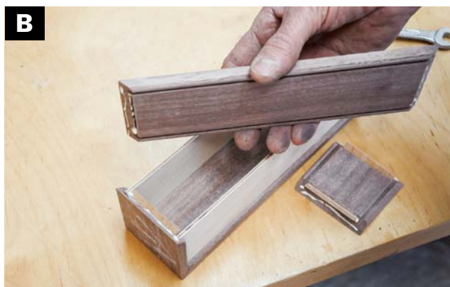
CAREFULLY ASSEMBLE the sides and ends around the Baltic-birch plywood bottoms.
