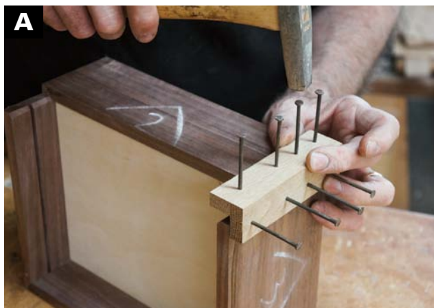
I MAKE A SIMPLE SHOPMADE MARKING GAUGE to mark the location of the dowel holes. You can also just mark them with pencil and awl to be ready to drill.
