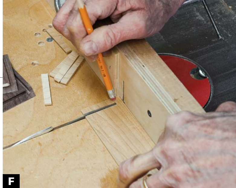
CUT THE SPLINE STOCK to exact length using the crosscut sled and stop block.
