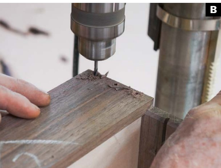
USE THE DRILL PRESS to drill the dowel holes.
