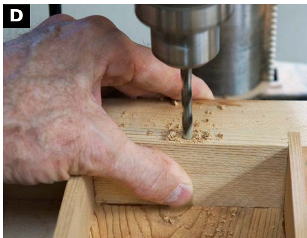
DRILL THE MATCHING HOLE in the box ends. Be sure to go deep enough for the length of the pin.
