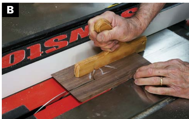
CUT THE FRONT PIECE to its smaller size to allow for the drawer.
