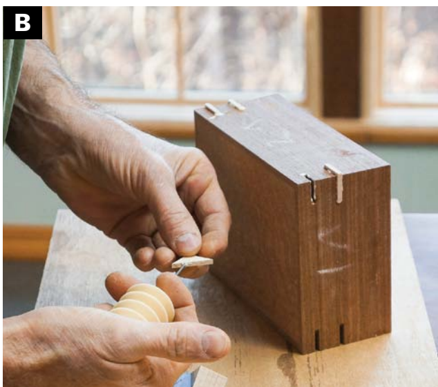
INSTALL AND GLUE all the keys in place.
