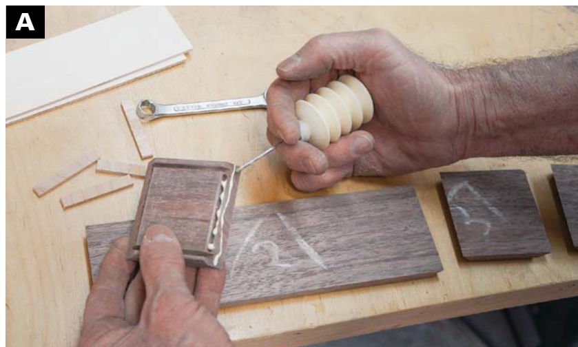
SPREAD GLUE in the grooves and on the surface of the miter joints.
