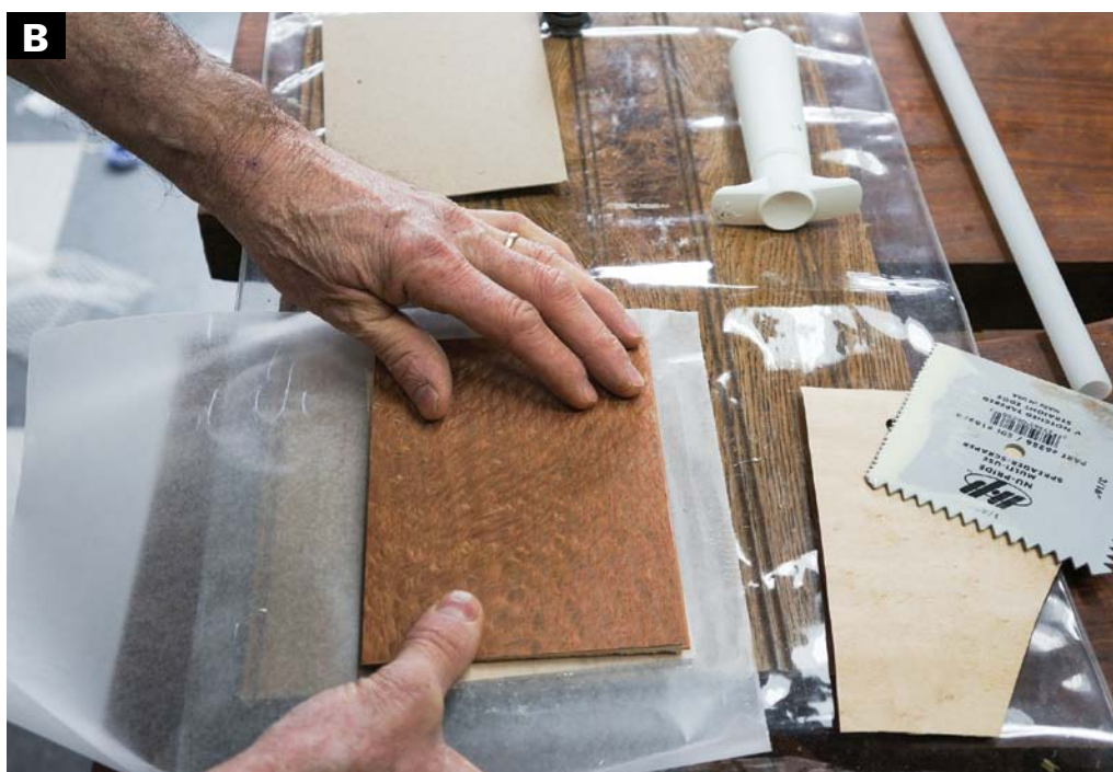
PRESS THE VENEER firmly in place. Wax paper can help to keep from getting glue where you don't want it.
