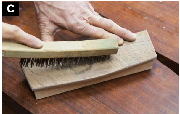
USE A WIRE BRUSH to remove loose material and fuzzy wood grain, while leaving the original saw marks and weathering.
