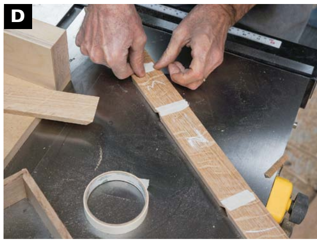
TAPE THE FRONT, back, and ends with masking tape, aligning the grain as it was in the original wood.
