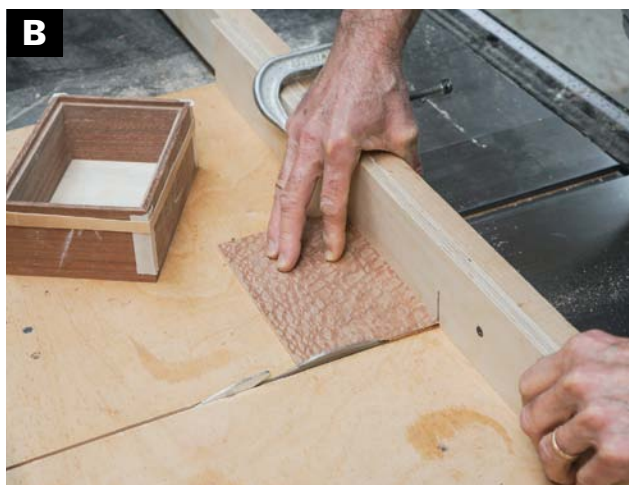
USE THE 90-DEGREE CROSSCUT SLED on the tablesaw to cut the veneered panel to fit.
