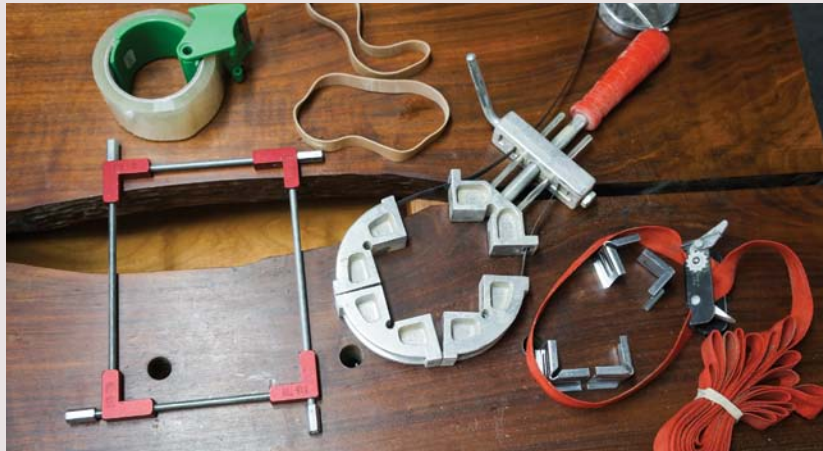
A VARIETY OF CLAMPING TOOLS work well for mitered corners. Clockwise from left: picture-frame clamp, clear tape, rubber bands, and band clamps.
