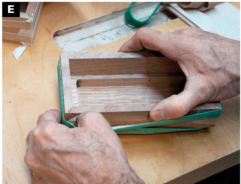
ASSEMBLE THE BOX SIDES around the box bottom, and use rubber bands to hold things tight while glue sets.
