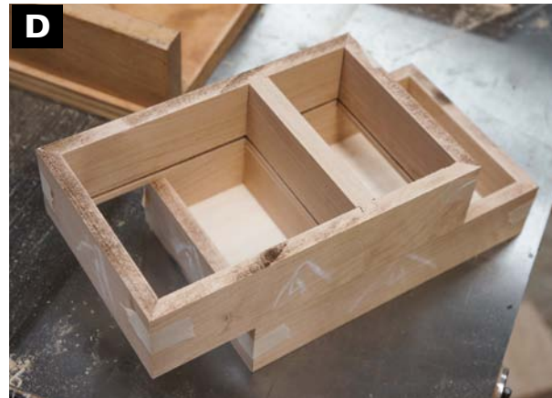
CUT THE BOTTOM panels to fit, proceed with assembly, and install the magnets at the center of each divider strip.
