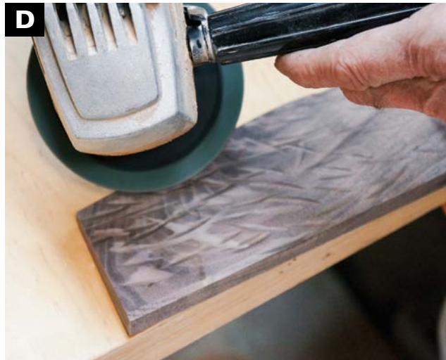
CREATE YOUR OWN TEXTURE to establish rhythm. An angle grinder with a 120-grit sanding disk can be applied in a rhythmic and varied texturing technique.
