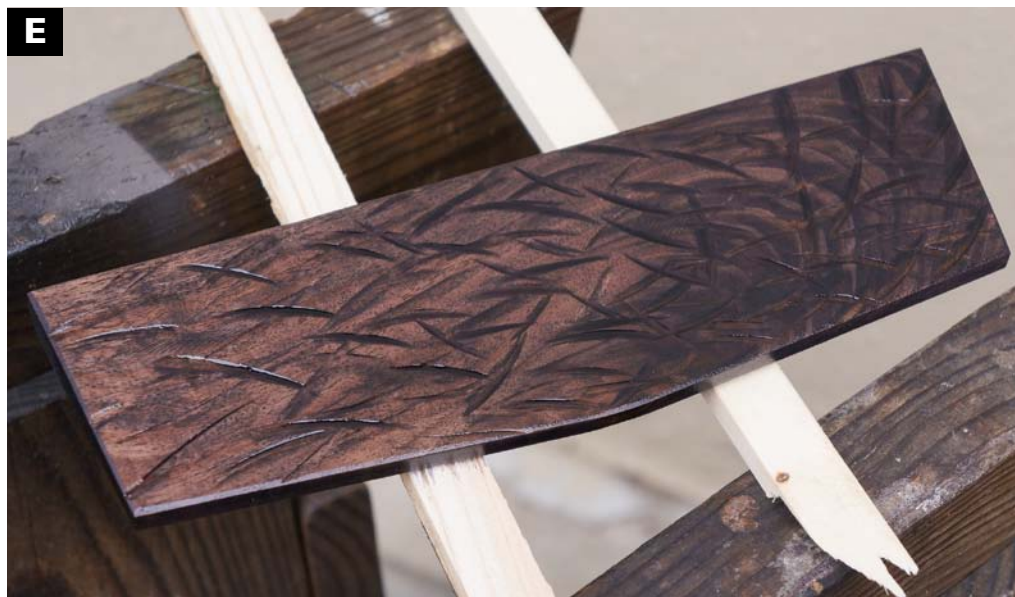
CREATE CONTRAST with stains and chemical treatments of wood. Apply ebonizing solution and watch walnut turn black.
