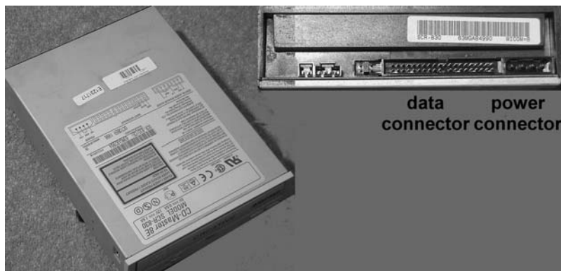
Figure 1.8 A CD-ROM drive as seen from above – the casing covers all of the internal structure so that there is no risk of laser light emerging
