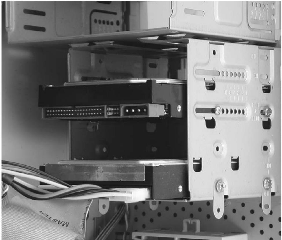
6. Connect a drive cable and a power cable to the drive.
