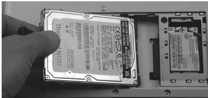
7. If the hard disk uses an enclosure, as in the example shown here, unscrew any retaining screws and then remove the disk from the enclosure. Insert the replacement disk, and then apply the retaining screws.
