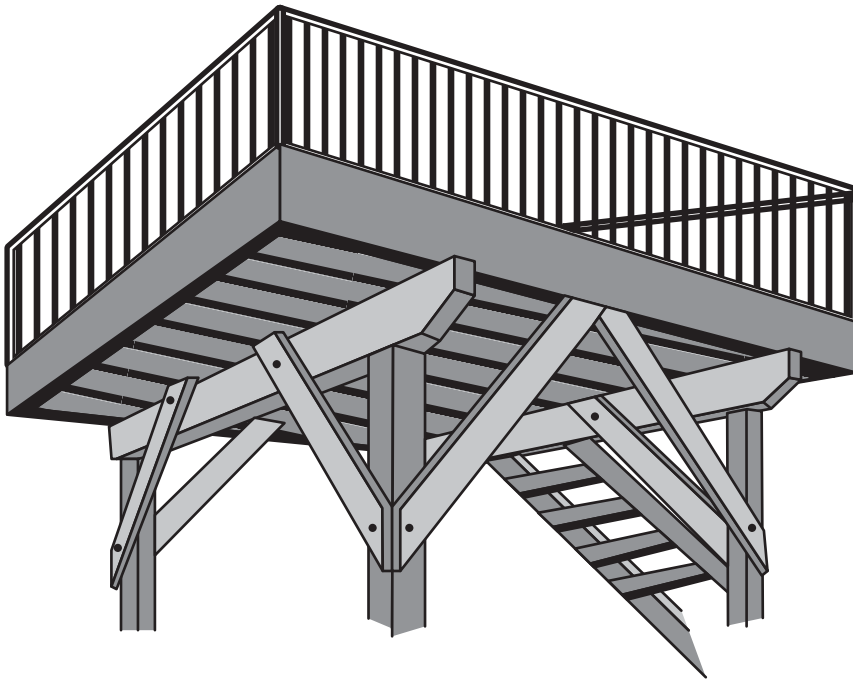
Fig. 6-21. Diagonal bracing on free-standing deck.
