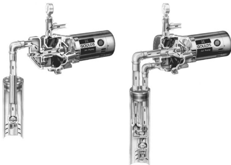
Fig. 13-13. Jet pumps: left—shallow-well jet pump, one pipe extending into well; right—deep-well jet pump, two pipes extending into well. Gould Pumps, Inc.
