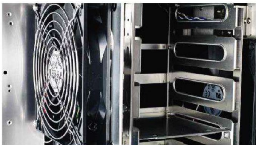
The use of 140mm fans on both sides of the hard drive cage ensures direct airflow to the core hardware despite the size of the case
