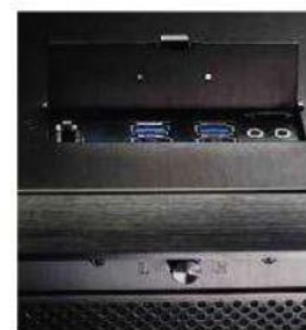
The front panel boasts four USB 3 ports, but the fan controller below it is poorly placed
