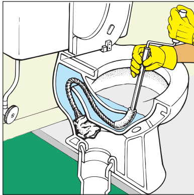
Figure 5-2: Using a toilet auger.
