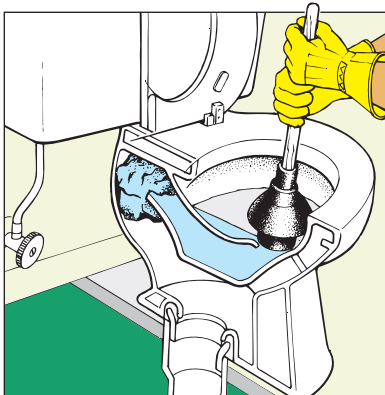
Figure 5-1: Positioning the plunger.
