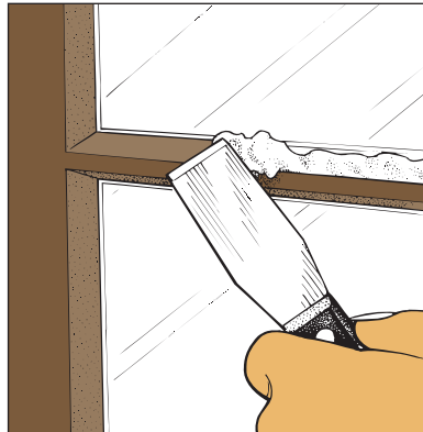
C. Drag the putty knife blade over the glazing putty at a 45 degree angle to smooth the putty. (Step 11)
