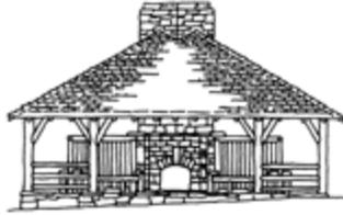
*A design for a shelter, taken from the design manual prepared for the Civilian Conservation Corps and the National Parks Service of the USA in the 1930s. The style is simple and robust, and uses materials as close to their natural state as possible: round logs, wooden shingles and rough stone all left to weather naturally.*
