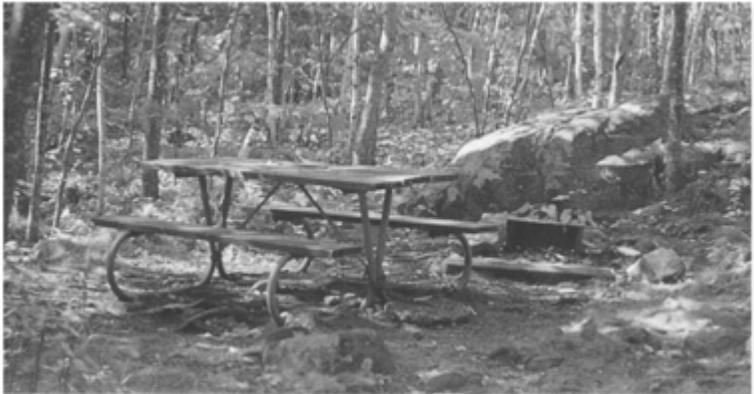
*An example of steel tubing for the frame and sawn wood planks for table and bench tops. This offers good leg-room for getting in and out. It fits surprisingly well into this wooded landscape, where the curve of the frame seems to echo the tree-trunks and branches. Acadia National Park, Maine, USA.*
