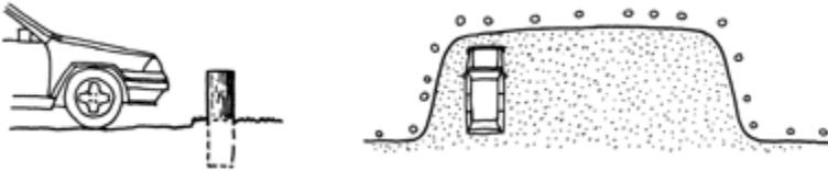
*This diagram shows the layout of log posts. Their spacing is important in order to prevent small vehicles from slipping in between them.*
