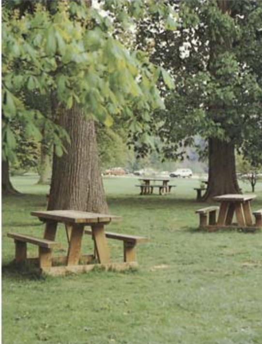
18 These picnic tables sit on the ground. They can be moved to avoid site damage, but they can also be stolen unless they are anchored. They may also be more difficult to place completely level on uneven ground.
