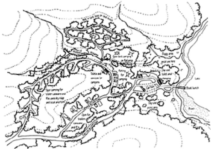
*This design for a large layout shows how terrain and vegetation can be used to provide a range of open and wooded sites for caravans/RVs or tents, together with a day-use area. Sensitive or difficult areas have been avoided, and circulation for pedestrians and vehicles has been organized.*
