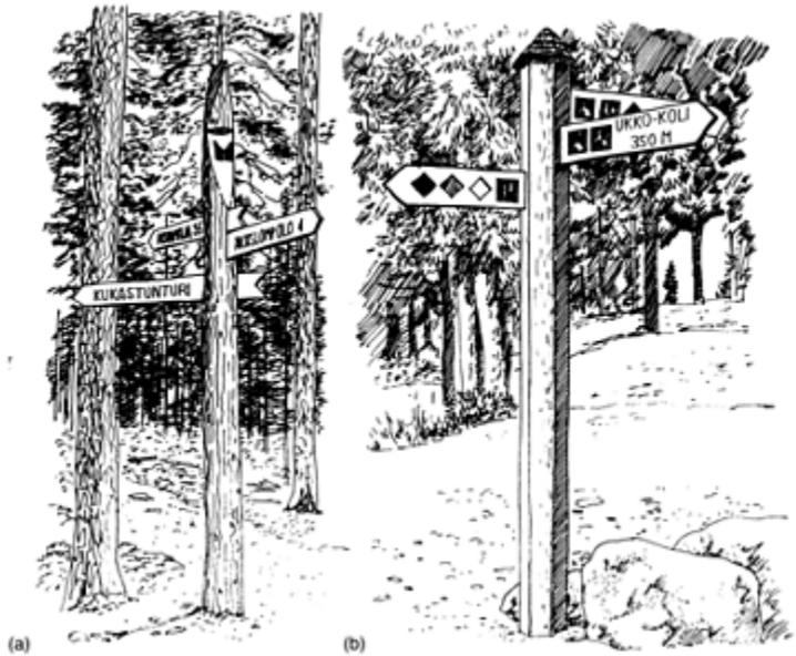
*In countries which get deep snow, short posts can be buried. Cross-country skiers need visible signs: (a) Arrow-shaped boards carrying the destination and route direction mounted in an upright post work well, and fit into the forest landscape. Finnish Lapland. (b) A fingerpost using colour-*
