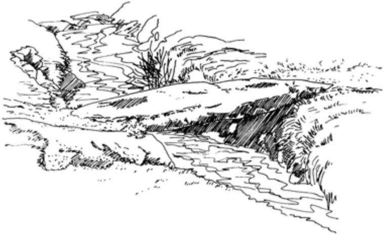
*A simple bridge for short spans: a stone slab laid across a narrow stream is ideal.
