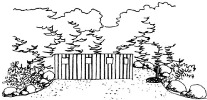
*A design for campsite utilities such as fire equipment, water, litter, grey water and chemical toilet disposal arranged into a neat enclosure provided with a lay-by and surfaced access. Trees and shrubs help to screen it, although the tidy design would also work in open sites.*
